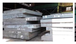
ASTM A588Grade K(A588GRK) Weather Resistant Steel Plate
