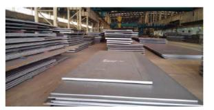
DIN17100 St37-3 Carbon Steel Plate
